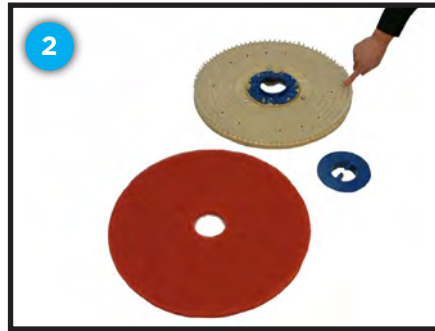
Disconnect center lock fitting & lay next to the pad driver
