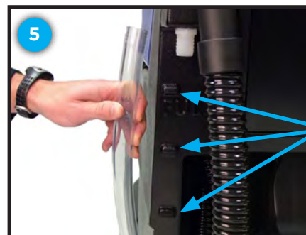
Sight gage hose released from press fitting
