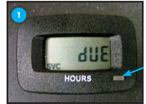
Hour meter showing "SVC DUE"
