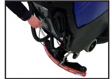
Lowering the squeegee assembly
