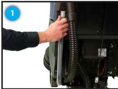
Check sight gage hose for solution level
