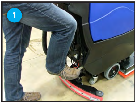
Lowering scrub head using foot pedal
