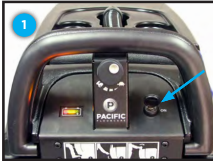
Turn unit on using key switch
