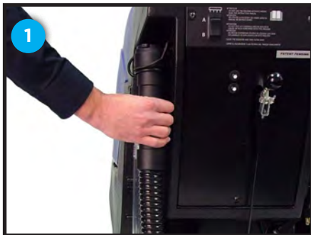
Recovery tank drain hose
