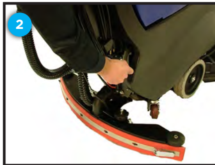
Locking in high down pressure setting by lifting foot lever
