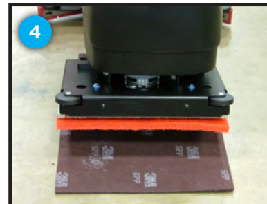
Place surface prep pad on floor in front of machine with backer pad
