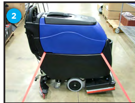
Tie down locations between recovery tank and solution tank
